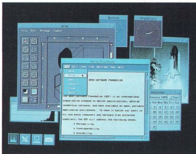
Photo 4: Motif features a distinctive three-dimensional look, while conforming to the X Window System and IBM's SAA interface standard.
